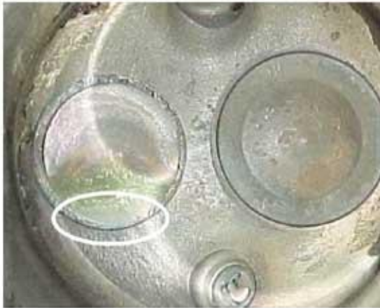
Burned exhaust valve. Note edge of valve face that has lost all combustion residue and striations moving toward center of valve.
